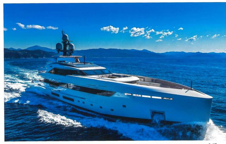
The naval architecture of the hull has been optimised for performance by Tankoa's Technical Office, based on an initial design by Massimo Visibelli, and the yacht has been built entirely in light aluminium alloy. Together, these features allow for a substantial reduction in fuel consumption. After the launch in February this year, the S501's first sea trials fully confirmed the design estimates and went far beyond
