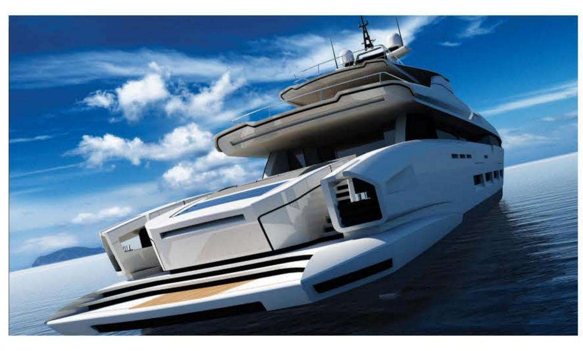
With a streamlined profile, the superyacht features two sprawling aft decks and open sundeck, which hosts a central bar and an al fresco dining area for up to 10 guests. Performance wise the vessel will be powered by a triple 2,683hp MTU engine set-up, twin Kamewa water jets and a central booster.
