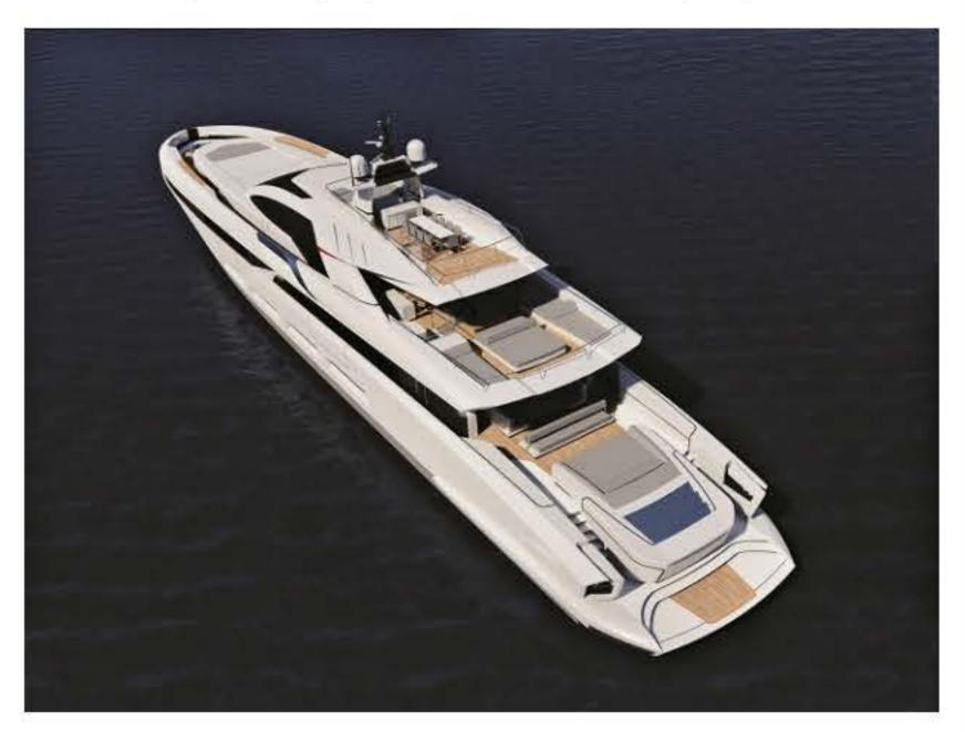
Equipped with three MTU 2,000kW diesel engines coupled to two Rolls-Royce Kamewa waterjets and a central booster, the all-aluminium yacht boasts a maximum speed of 28/30 knots at half load.
