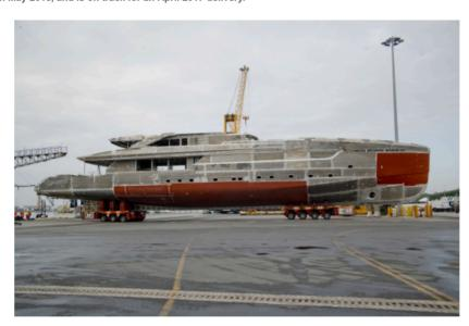
The yard reports that the vessel's aluminium hull and superstructure is complete with the fairing process currently underway. The interior has been approved by the owner and is now being constructed for installation. The yacht's engines that will provide a range of 5,000 nm at 12 knots and a top speed of 16 knots, have already
